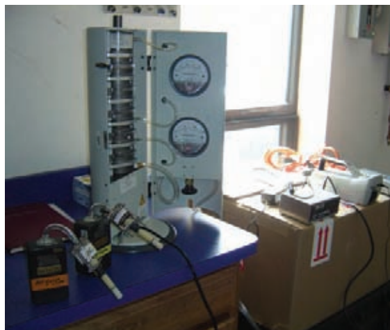
Figure 7–1. Examples of different sampling instruments used to measure occupational exposures to nanoparticles including the determination of real-time particle number concentrations and size-fractionated mass concentrations
